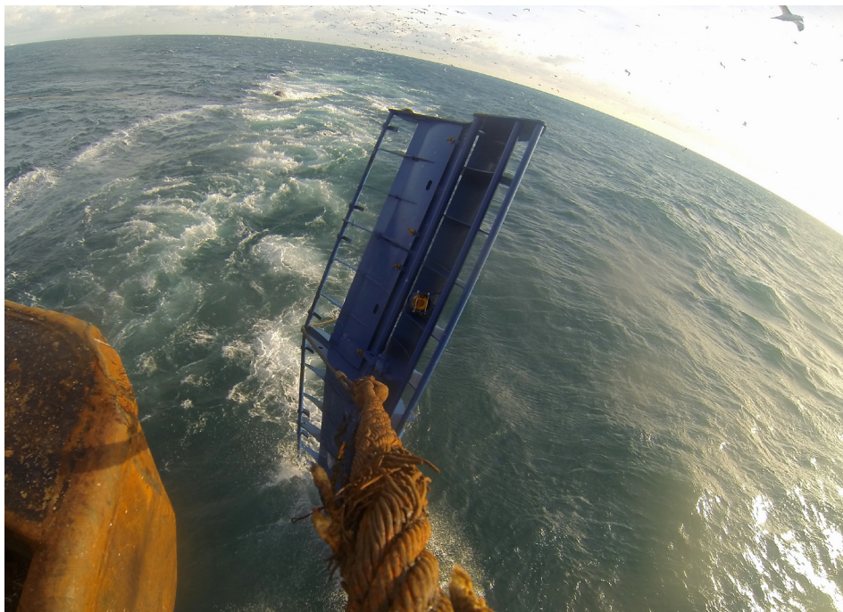
The "Cornelis Vrolijk" is the first vessel to use the "Flipper" doors. Here the door is seen in action with the foils released - reducing the doors surface area. Photo: Cornelis Vrolijk.
